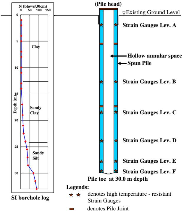
Fig. 1. Diagrammatic illustration of conventional spun pile instrumentation scheme
