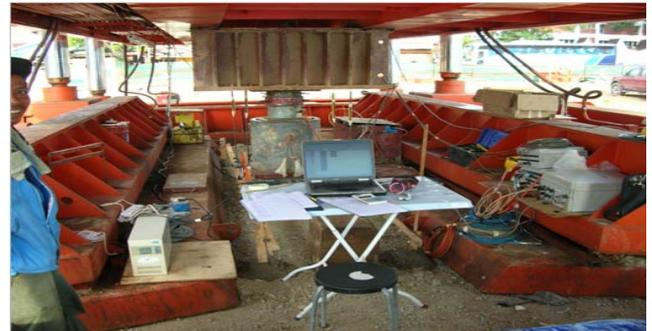
Fig. 7. Instrumentation and monitoring test set-up for Test Pile 1 at Melaka site, Malaysia
