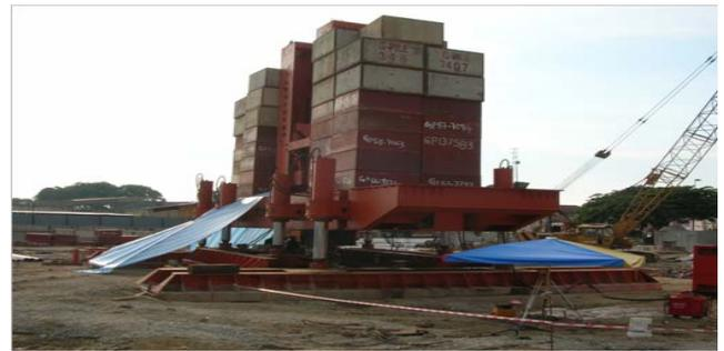
Fig. 6. Static axial compression load test set-up for Test Pile 1 at Melaka site, Malaysia
