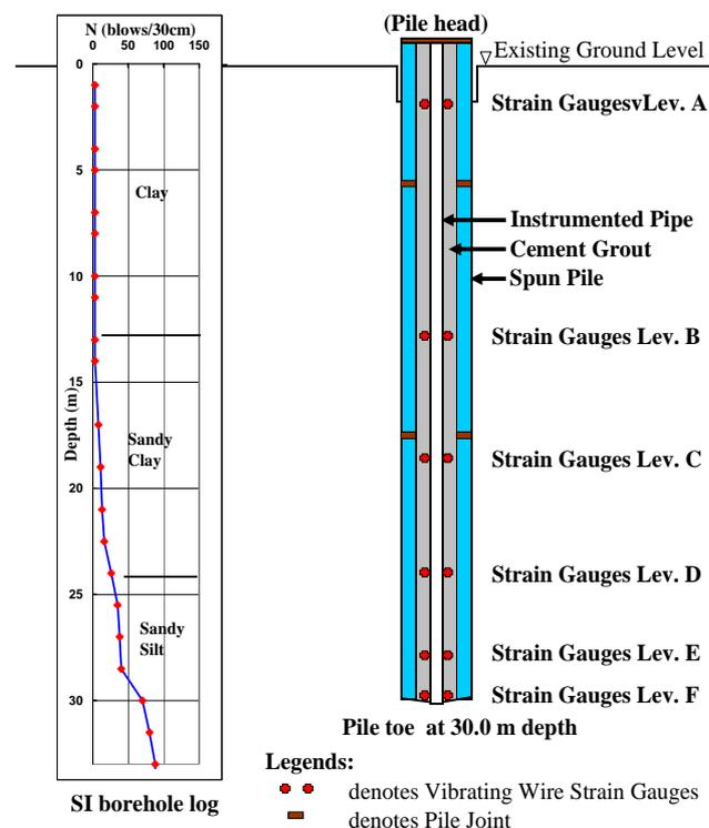
Fig. 2. Diagrammatic illustration of approximate instrumentation scheme. As this approximate method is generally more “convenient” to be implemented than the conventional
