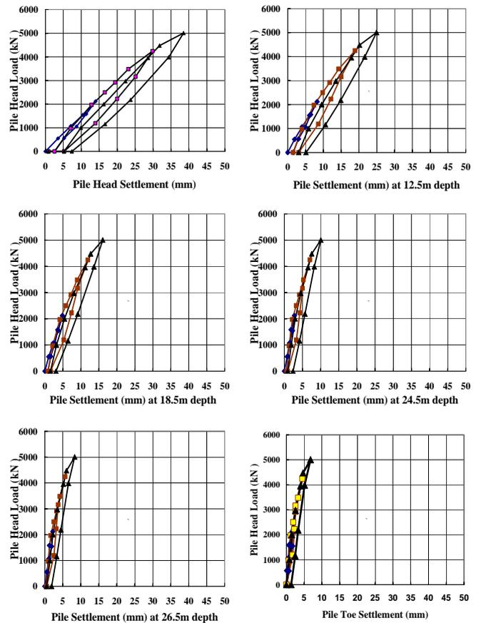
Fig. 8. Pile head settlement and pile settlement at various depths including pile toe for Test Pile 1 at Melaka site, Malaysia
