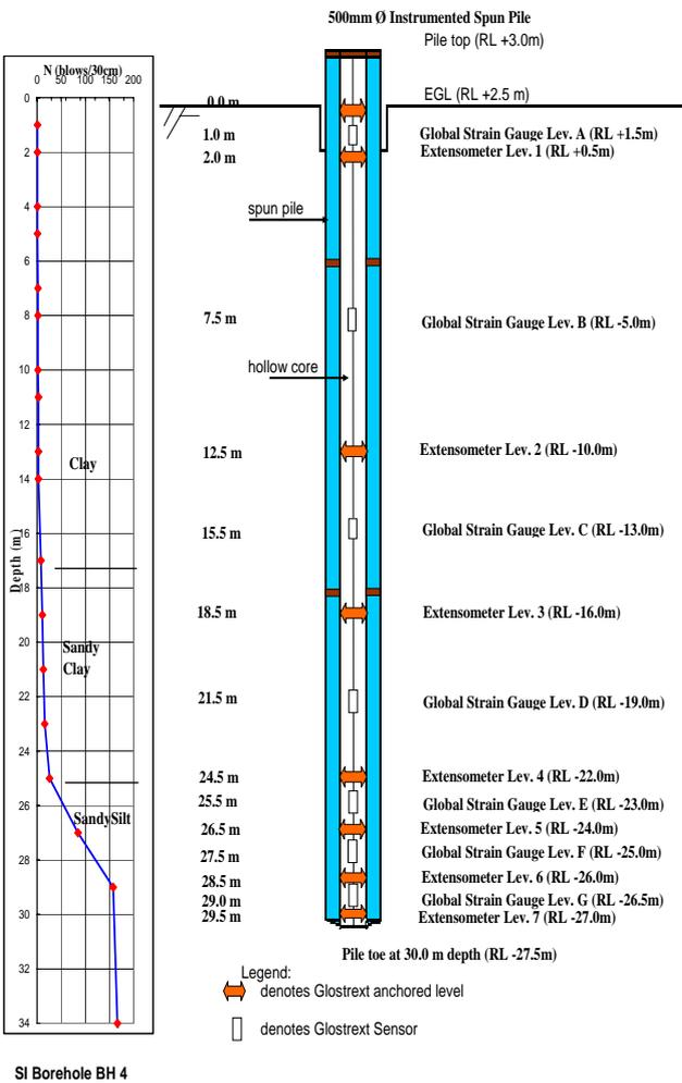
Fig. 5. Test Pile 1 instrumentation using global strain
