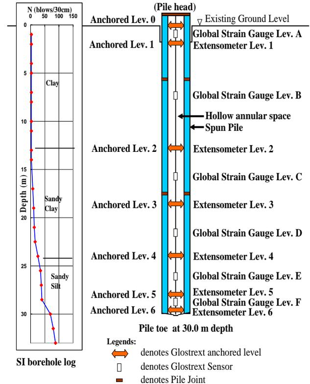
Fig. 4. Schematic diagram of typical instrumented spun pile using global strain extensometer technology
