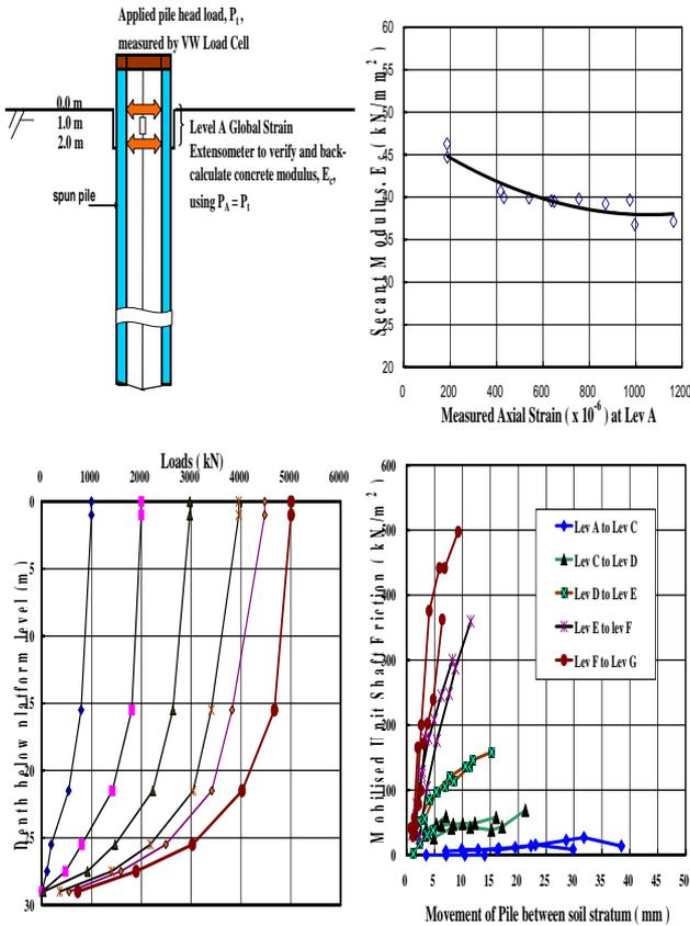
Fig. 9. Level A sensor arrangement for verifying and back-calculate  $E_c$  values, modulus-strain curve, load distribution curve and mobilized unit shaft friction versus average movement of pile between soil stratum measured using global strain extensometer for Test Pile 1
