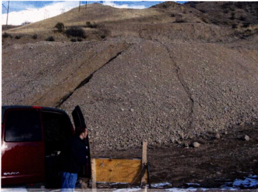
**Figure 12a.** View of the experimental site. Gravel pile used to simulate a mine highwall.
