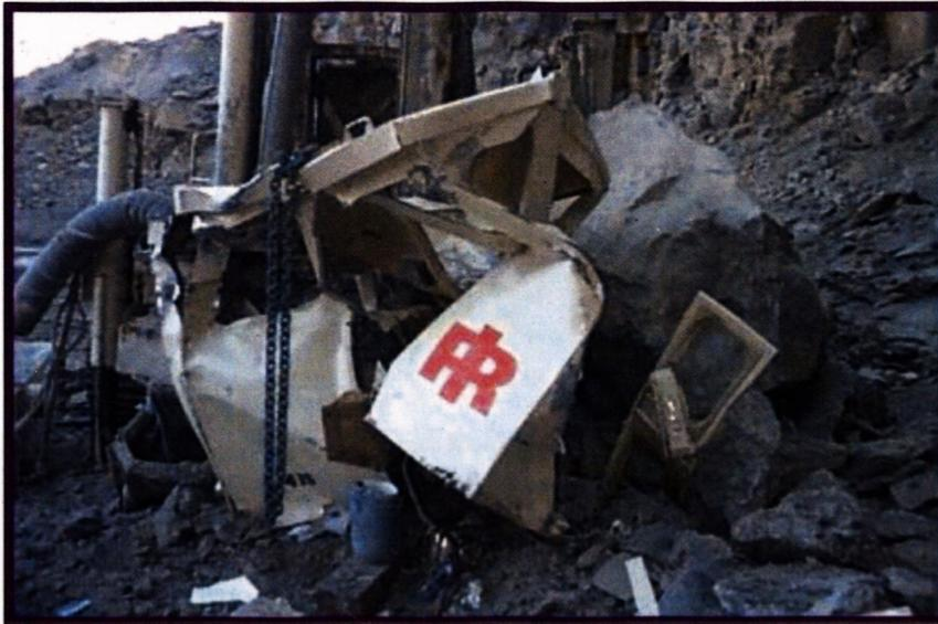
**Figure 8.** Drill cab crushed and operator fatally injured from highwall failure at open pit mine. Photo from Mine Safety and Health Administration (MSHA, 1998).
