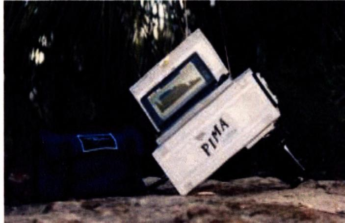
**Figure 5.** Field-portable point spectrometer. (Photo courtesy of Integrated Spectronics [Cocks, 2003]).
