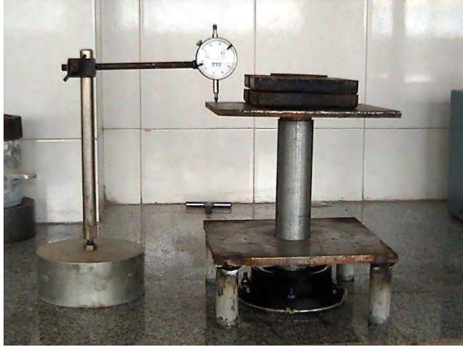
Fig. 7 How to apply Stress to Measure Swelling Pressure by using the Instrument shown in Figure 4
