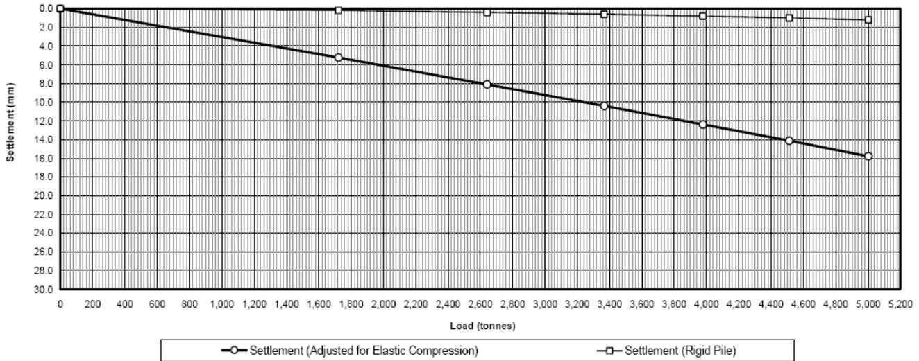
Figure 12: Equivalent Top Load vs. Settlement Chart
