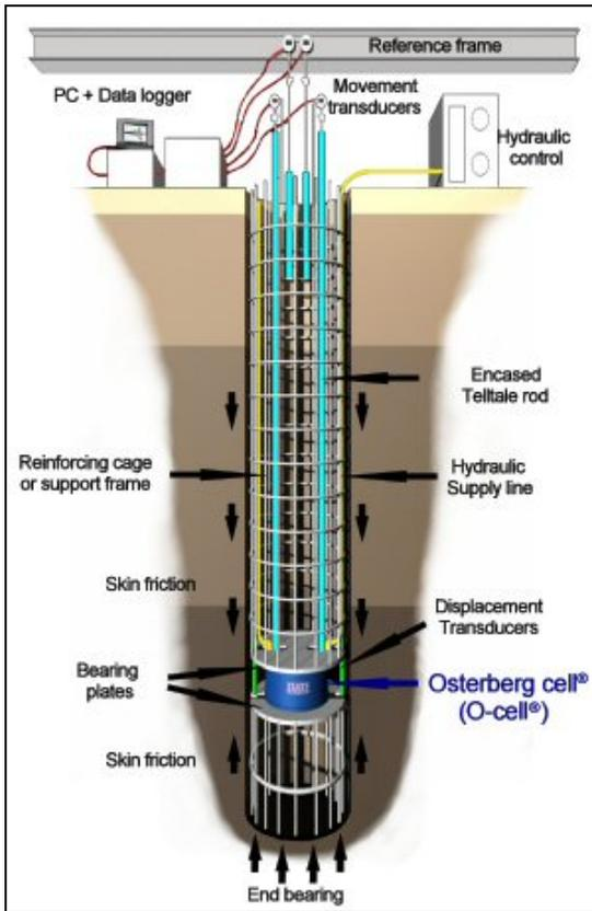
Figure 4: Typical Osterberg Load Cell Setup
