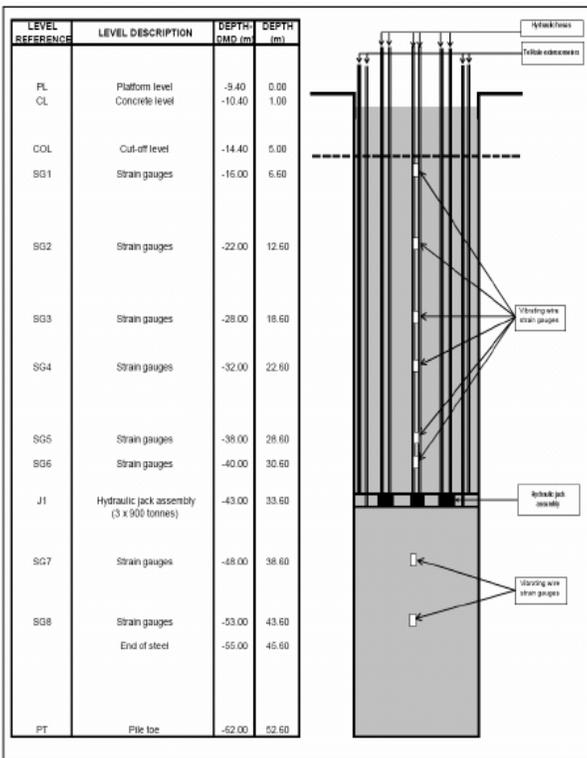
Figure 11: Test Pile and Testing System Geometry
