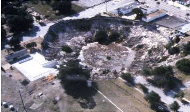
Fig. 1. 100 m wide and 30 m deep sinkhole in Winter Park, Florida, USA, 1981.
