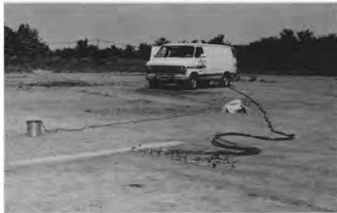
Fig. 10 - Test Setup of Passive Isolation by a Concrete Trench (Site 3 with barrier)
