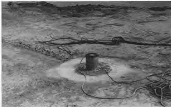
Fig. 9 - Test Setup of Active Isolation by a Concrete Trench (Site 2 with barrier)
