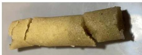
**Figure. 13—Portion of the sand/gel removed from the sandpack.**
