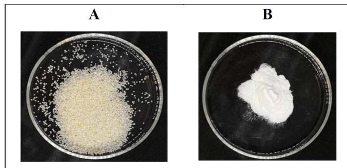
Figure. 1—(A) Proppant quartz sand of 20/30 mesh and (B) Micro-sized RPPG of 170/230 mesh.
