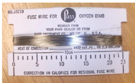
A.21: Calibrated Fuse Wire for Oxygen Bomb Calorimeter
