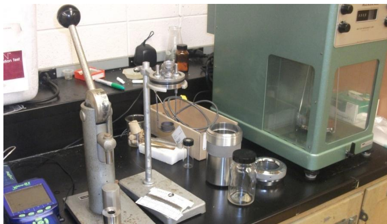
A.23: Configuration of Cucumber Sample in Bomb Calorimeter
