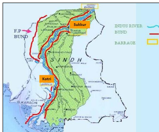
Fig.16. Flood Protective embankments shown in red color along River Indus in southern part of Indus Basin (WAPDA Report, 2010)
