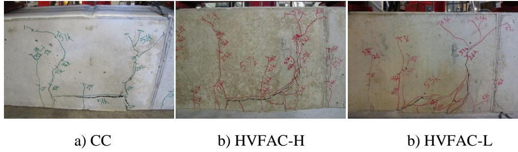
Figure A. 4 - Crack pattern of the beams at bond failure
