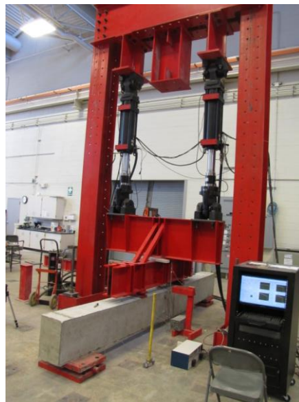
c) Splice test setup with specimen loaded
