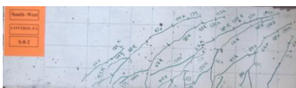
Figure 3 - Crack pattern of the beams at shear failure (Study B)
