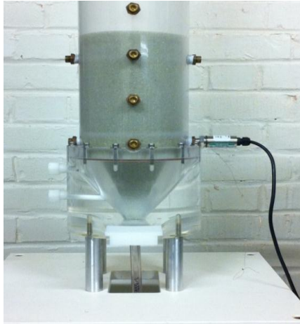
Figure 4.3. Pressure transducer applied for measurement on 0.152 m ID spouted bed
