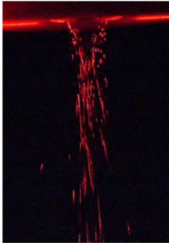
Figure 3: Typical image of the powder stream taken by digital camera
