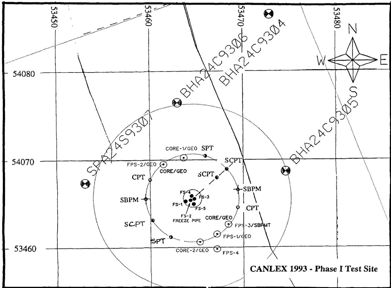
Figure 5. Phase I site plan showing test locations.
