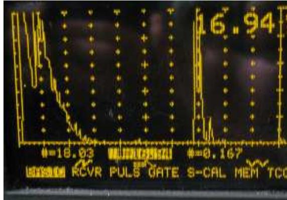
(b) Ultrasonic Graph of a Laser Deposited Ti-6Al-4V Specimen
