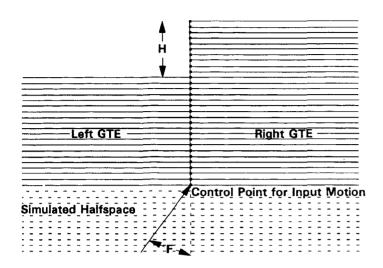
Figure 2: Stepped halfspace model for inclined wave incident on a vertical slope.
