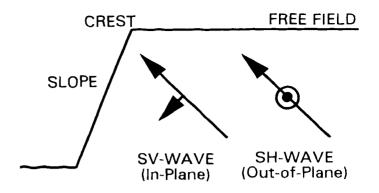
Figure 1: Definition of wave types.
