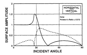
Figure 11: Variation of surface amplitude with incident angle.
