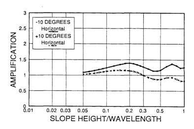
Figure 4: Amplifications at the crest for inclined SH-wave incident on a vertical slope,  $F = -10^{\circ}$  and  $+10^{\circ}$ ,  $\beta = 1\%$ .
