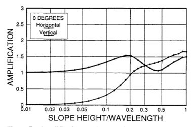
Figure 7: Amplifications at the crest for inclined SV-wave incident on a vertical slope,  $F = 0^{\circ}$ ,  $\beta = 1\%$ .
