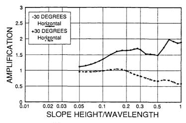
Figure 6: Amplifications at the crest for inclined SH-wave incident on a vertical slope,  $F = -30^{\circ}$  and  $+30^{\circ}$ ,  $\beta = 1\%$ .
