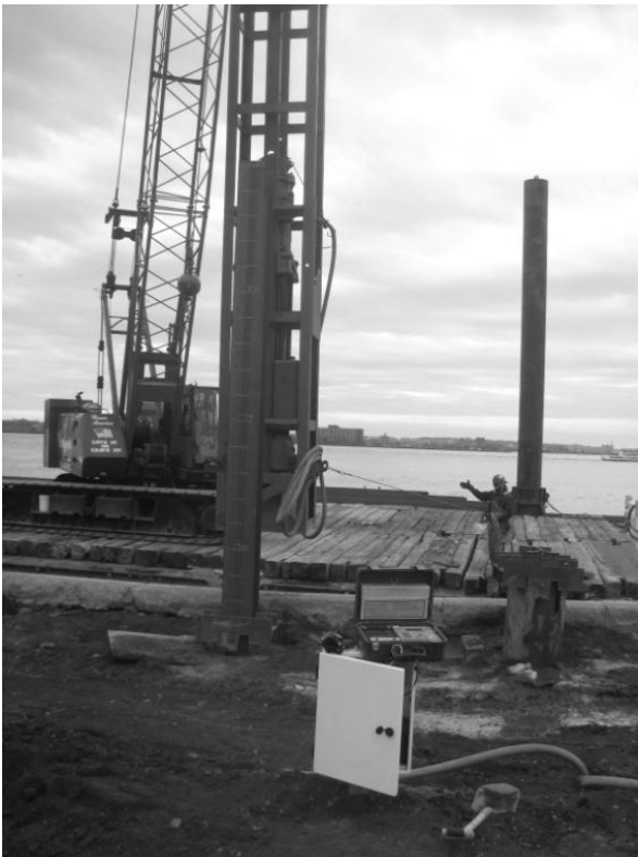
Fig 5. Vibration monitoring enclosing box with Blastmate seismograph.
