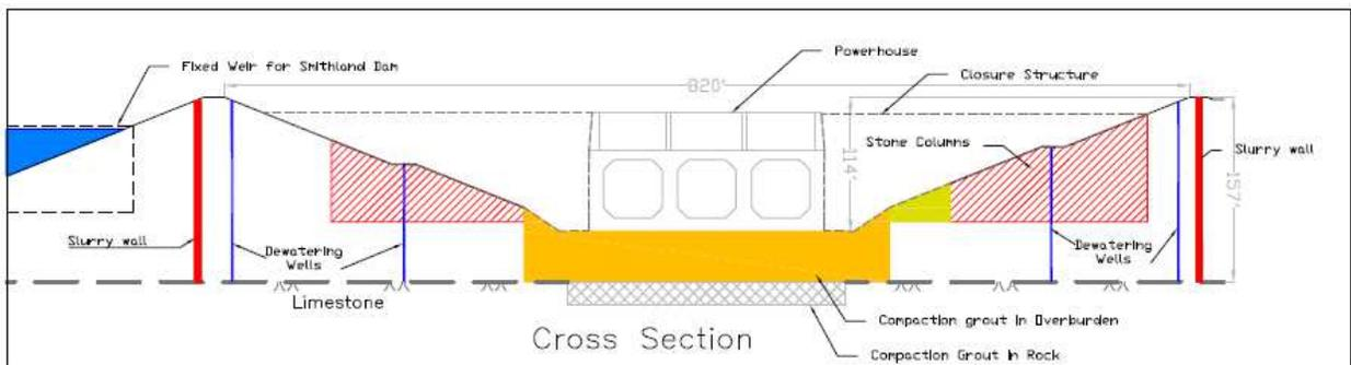
Fig 5. Cross Section of Ground Improvement
