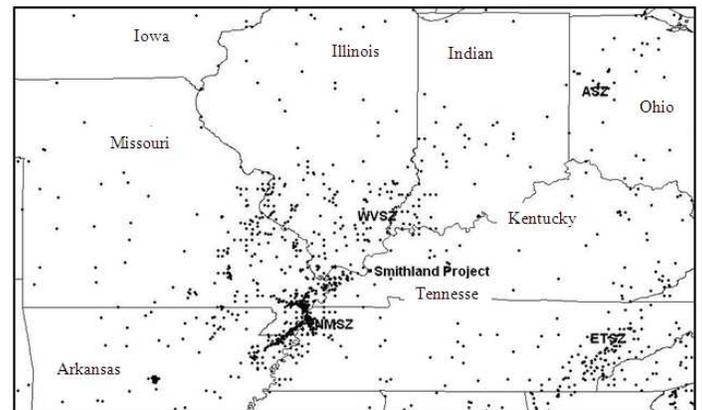
Fig.3. Seismicity of the Central and Eastern United States
