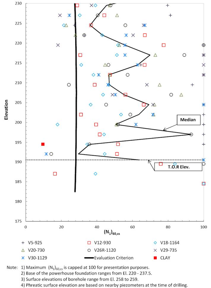
Fig. 9. Post-Treatment Results for Southwest Section in Powerhouse Foundation
