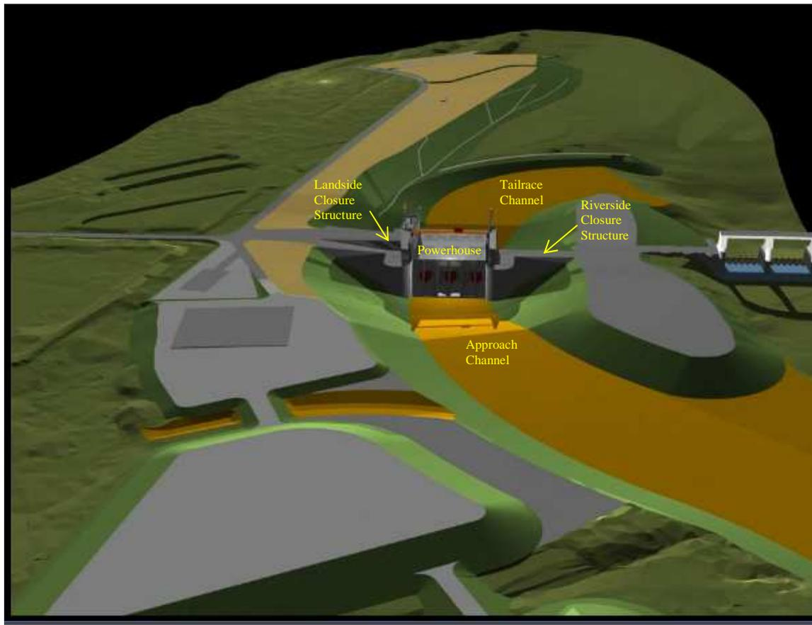
Fig.2. Project Components of Smithland Hydroelectric Project
