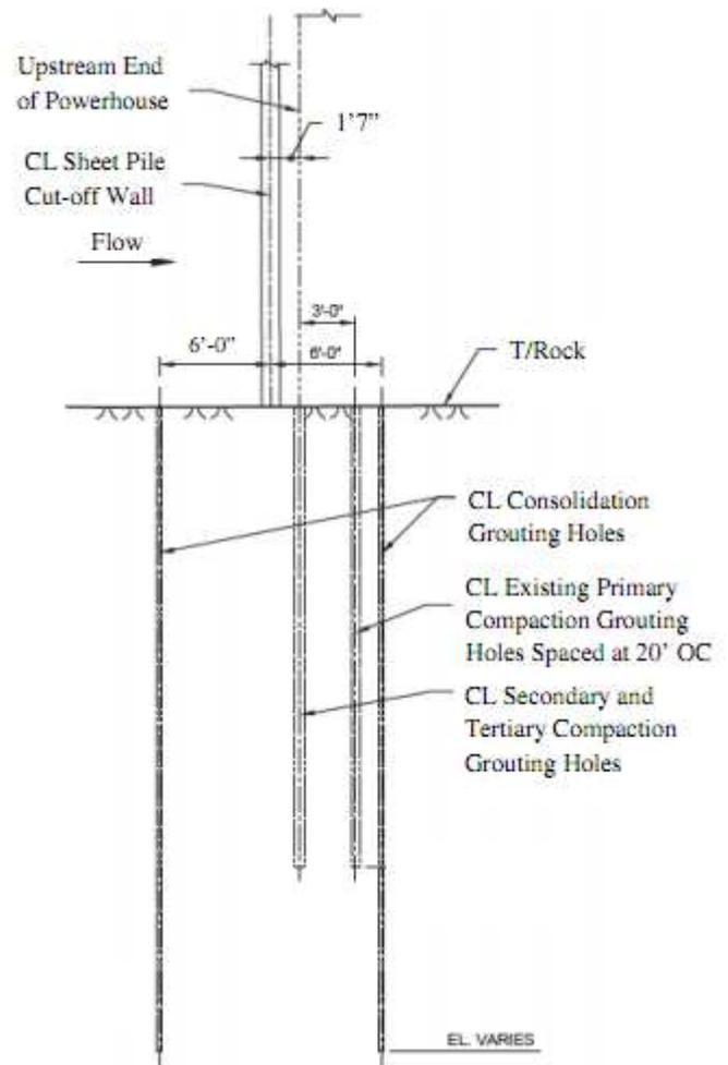
Fig. 6. Cross section of Consolidation Grouting Along Cut-off Wall
