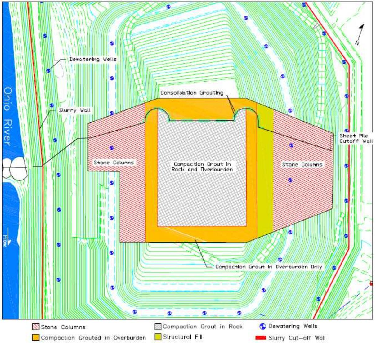
Fig 4. Plan View of Limits of Ground Improvement
