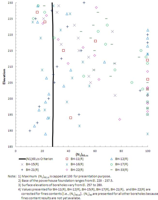
Fig. 8. Pre-Treatment Results for Powerhouse Foundation
