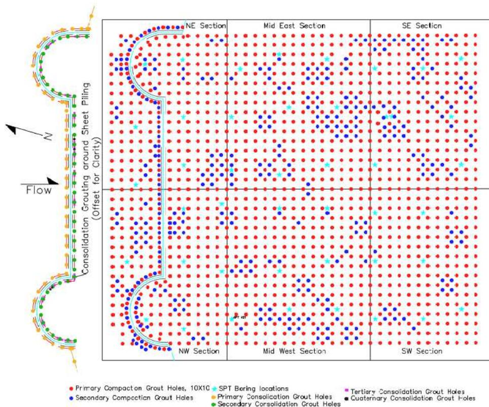
Fig. 7. Layout of Compaction Grouting Holes in the Footprint of Powerhouse and Cut-Off Wall
