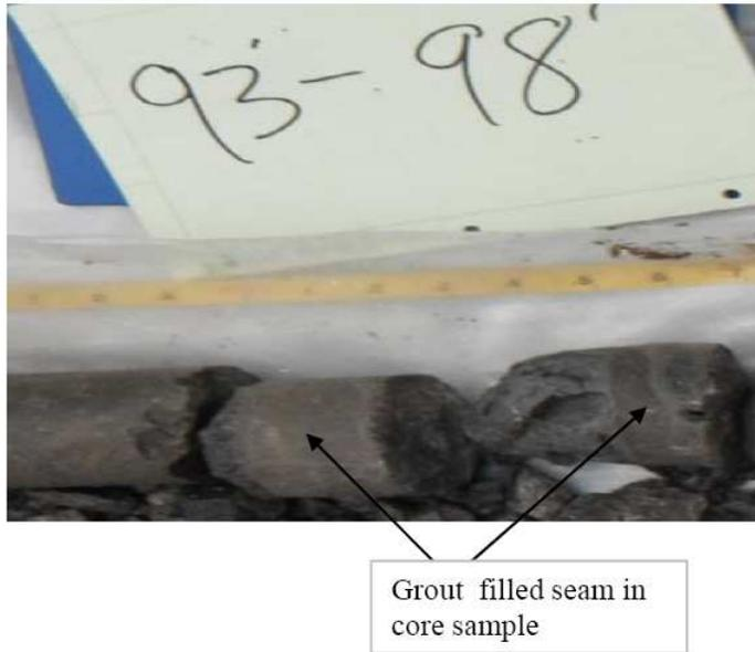
Fig.9 Grout-Filled Seams in Core Sample
