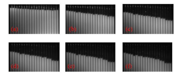
Figure 12. Measurement of water relative permeability from drainage process in 500nm deep nanopores. (a)~(f) are images of nanopores at different time with interval of 20 seconds.
