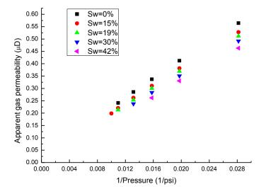
Figure 13. Gas slippage effect at different water saturations.
