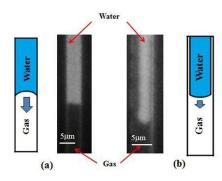
Figure 6. Water displacing gas patterns, two different interface patterns. (a) Frontal displacement interface under pressure drop of 12.5psi; (b) Liquid plug with cavity under pressure drop of 0.8 psi.
