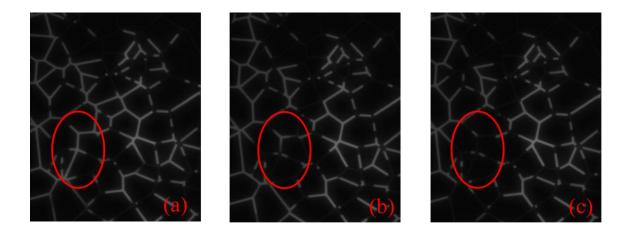
Figure 4. Haines jumps for drainage process in 300nm deep network nanopores.
