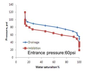
Figure 10. Relationship between capillary pressure and water saturation for drainage and imbibitions processes in 300nm deep network nanochannels.
