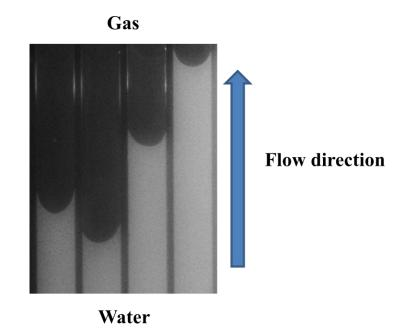
Figure 5. Piston-type motion for imbibition process in 500nm deep nanopores.
