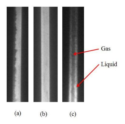
Figure 4. Water/gas two phase flow patterns. (a) Stratified flow; (b) Single phase flow; (c) Annular flow.
