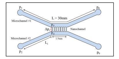
Figure 2: Top view of nanofluidic chip and pressure control.
