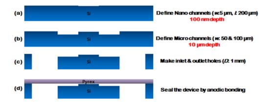
Figure 3: Cross-sectional schematic of Si-Pyrex micro- and nano-channel fabrication process.
