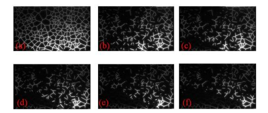
Figure 14. Measurement of water relative permeability from drainage process in 300nm deep network nanopores. (a)~(f) are images of nanopores at different time with interval of 60 seconds.
