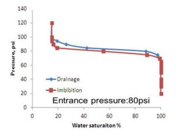
Figure 11. Relationship between capillary pressure and water saturation for drainage and imbibitions processes in 100nm deep nanochannels.
