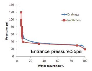
Figure 9. Relationship between capillary pressure and water saturation for drainage and imbibitions processes in 500nm deep nanochannels.
