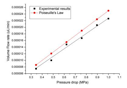
Figure 3. Average volume flow rate vs. pressure drop in a nanochannel.
