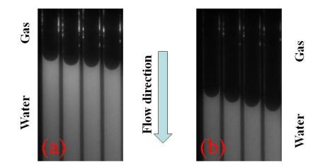
Figure 2. Piston-type motion of drainage process in 500nm deep nanopores.
