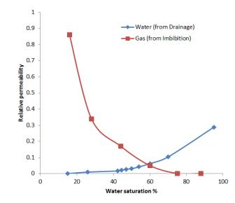
Figure 15. Relative permeability of the wetting and non-wetting phase with respect of wetting phase saturation in 300nm deep network nanopores.
