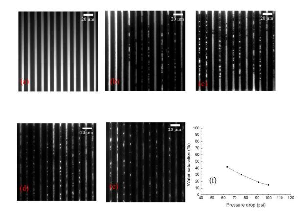
Figure 9.Water saturation during gas displacing water. (a) Image of 100% water saturation; (b) Image of 42% water saturation; (c) Image of 30% water saturation; (d) Image of 19% water saturation; (e) Image of 15% irreducible water saturation; (f) Water saturation under various pressure drop.
