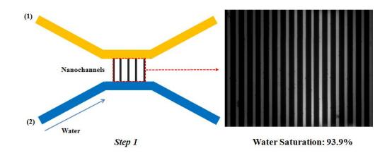
Figure 10. Step 1 - Measurement of gas permeability at different water saturations.
