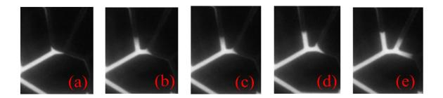
Figure 8. Cooperative filling for imbibition process in 300nm deep network nanopores.
