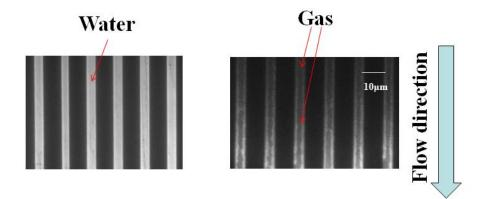
Figure 3. Annular-type flow of drainage process in 100nm deep nanopores.
