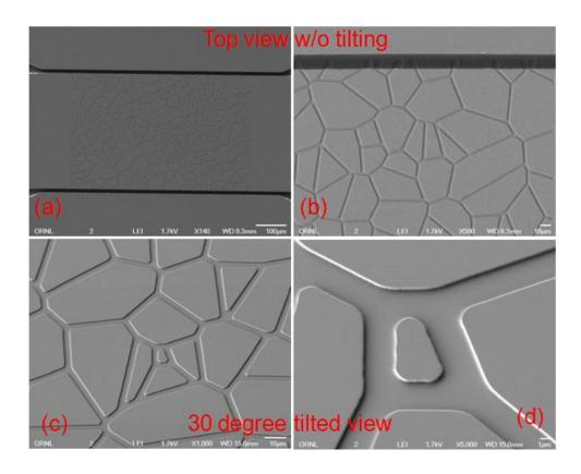
Figure 1. SEM images of fabricated random network nanopores. (a) An overview of microchannels and nanopores from top; (b)~(d) enlarged SEM images of nanopores with  $3\mu m$  width and 300nm depth.
