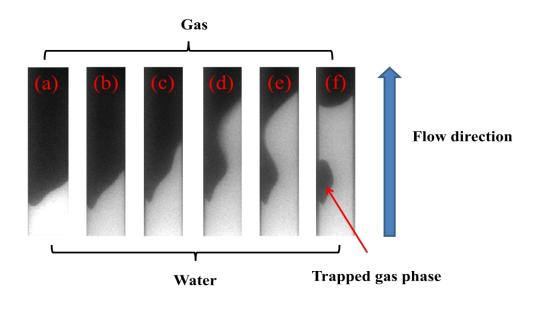
Figure 6. Local "snap-off" for imbibition process in 500nm deep nanopores.
