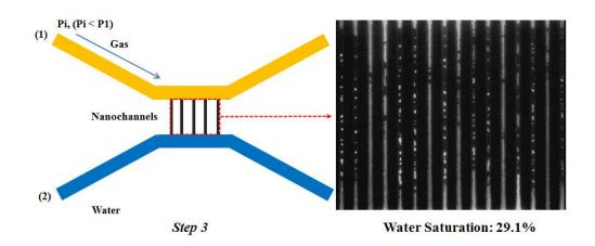
Figure 12. Step 3 - Measurement of gas permeability at different water saturations.
