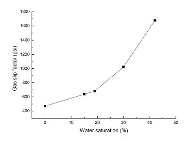
Figure 14. Correlation between water saturation and gas slippage factor.
