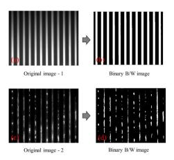
Figure 5: Image processing. (a) Original image of 100% water saturation in nanochannels; (b) Binary Black/White image of (a); (c) Original image of remained water saturation in nanochannels; (d) Binary Black/White image of (c).
