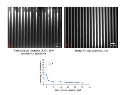
Figure 7. Gas saturation during water displacing gas. (a) Remained gas saturation in nanochannels after spontaneous imbibition; (b) Irreducible gas saturation in nanochannels; (c) Remaining gas saturation under various water injection pressures.
