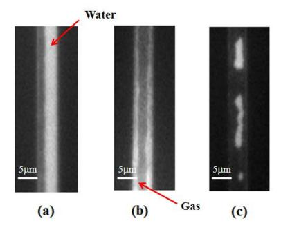
Figure 8. Flow patterns of immiscible two-phase flow in nanochannesl. (a) Side flow of gas; (b) Annular flow; (c) Water slug.
