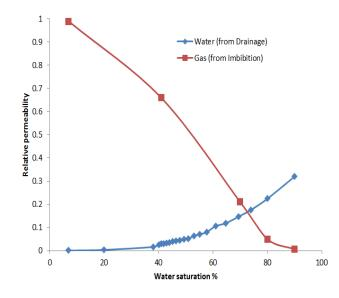
Figure 13. Relative permeability of the wetting and non-wetting phase with respect of wetting phase saturation in 500nm deep nanopores.
