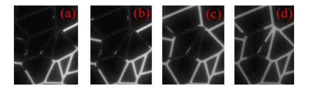
Figure 7. Snap-off for imbibition process in 300nm deep network nanopores.
