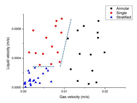
Figure 5. Water/gas two phase flow regime map in nano-scale channels.
