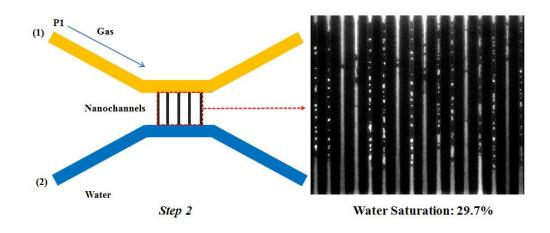
Figure 11. Step 2 - Measurement of gas permeability at different water saturations.
