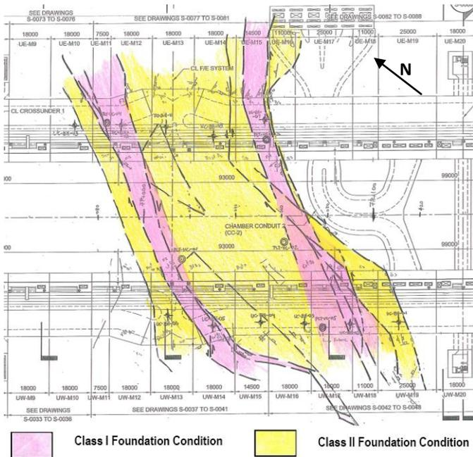
Fig. 5. Engineering Classification Map of LUC Fault Zone
