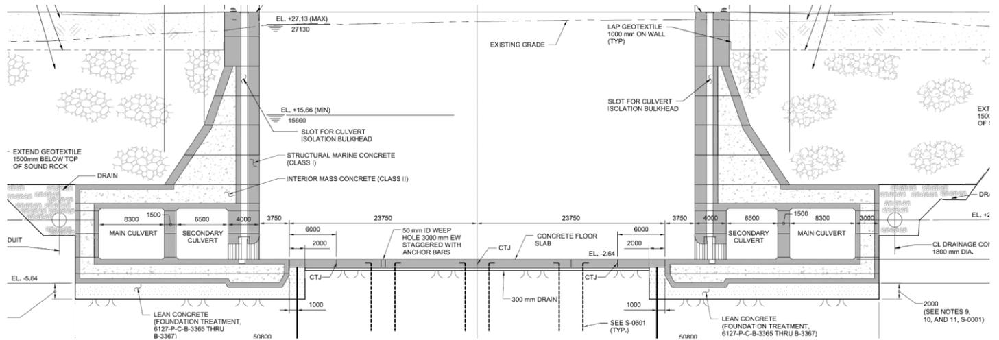
Fig. 13. Fault Zone Foundation Treatment including Lean Concrete and Chamber Floor Slab
