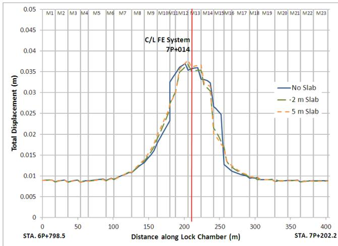
Fig. 8. Total Foundation Deformations at EOC (2D model)
