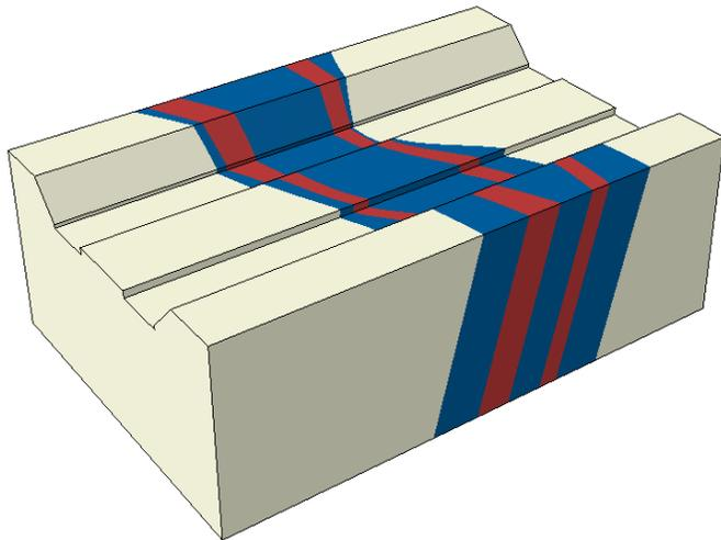
Fig. 10. Foundation including fault zone (3D model)
