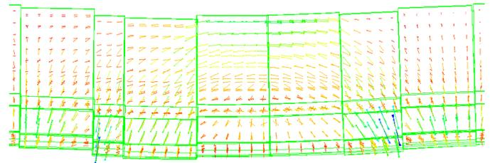
Fig. 11. Wall Arching Effect (deformations exaggerated for affect)
