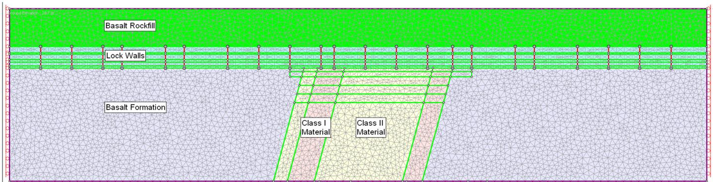
Fig. 7. 2D Model Layout of East Lock Wall Section (view looking east)
