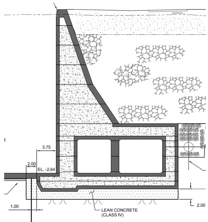
Fig. 6. Typical Lock Wall Section Modified for Fault Zone
