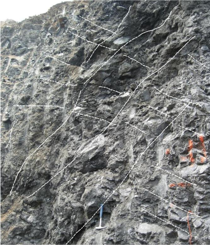
*Fig. 3. Cataclastic Basalt. Persistent and very close joint spacing intersected by steeply dipping shear planes.*
