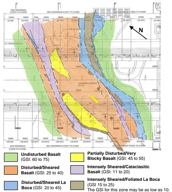
Fig. 2. Geologic Map of LUC Fault Zone
