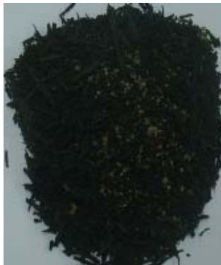
Figure 4. Magnified view of sand and 50% shredded rubber tire mixture.
