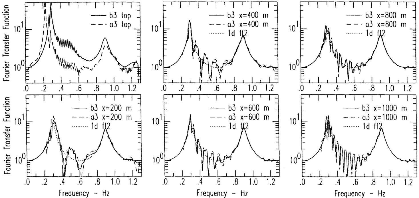
**Figure 4** : Fourier transfer functions at building top and various surface sites, from  $x=200$  m to  $x=1000$  m, for models b3 (solid line) and a3 (dashed line). Surface responses are also with the 1D response of a single clay layer (dotted line).
