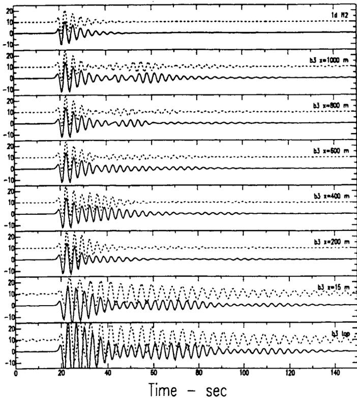
**Figure 5 :** Synthetic seismograms at building top (bottom trace) and 6 surface sites (from  $x=15$  m to  $x=1$  km) for model b3. The input signal is a Ricker wavelet having a characteristic frequency  $f_p = 0.28$  Hz. (Also compared with the 1D response of a single clay layer shown on top, and with the synthetics obtained with models a3, shown in dotted lines).
