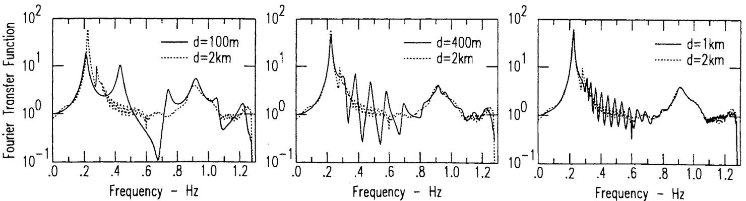
**Figure 6 :** An example of the effect of building spacing on the building response: the three diagrams compare the roof motion for different building spacings ( $d = 100$  m,  $d = 400$  m and  $d = 1$  km, respectively), with the roof motion for  $d = 2$  km (dotted line).
