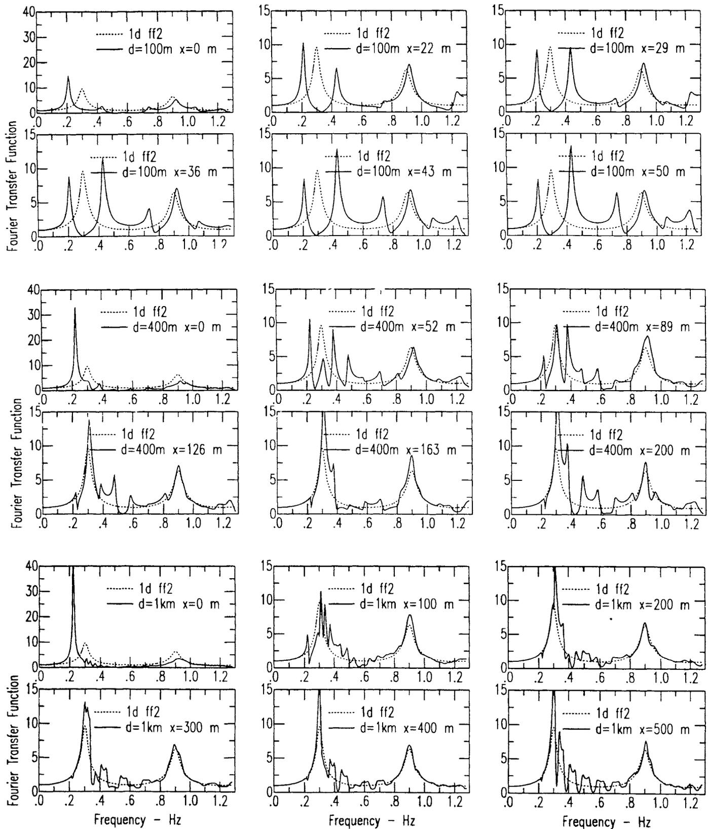
**Figure 7 :** An example of the effect of building spacing on the surface motion. For three different building spacings ( $d = 100\text{ m}$ ,  $d = 400\text{ m}$  and  $d = 1\text{ km}$ , respectively), the Fourier transfer functions of motion are displayed for 6 surface sites, located from building base to half-way between buildings, and compared with the 1D free-field response of the surface layer without buildings (dotted line)
