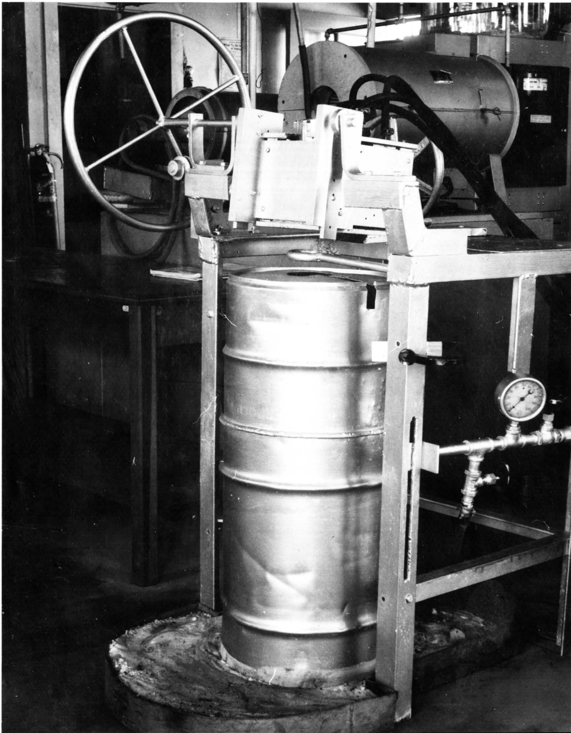
Figure 1 Blowing Apparatus for Making Metal Shot
