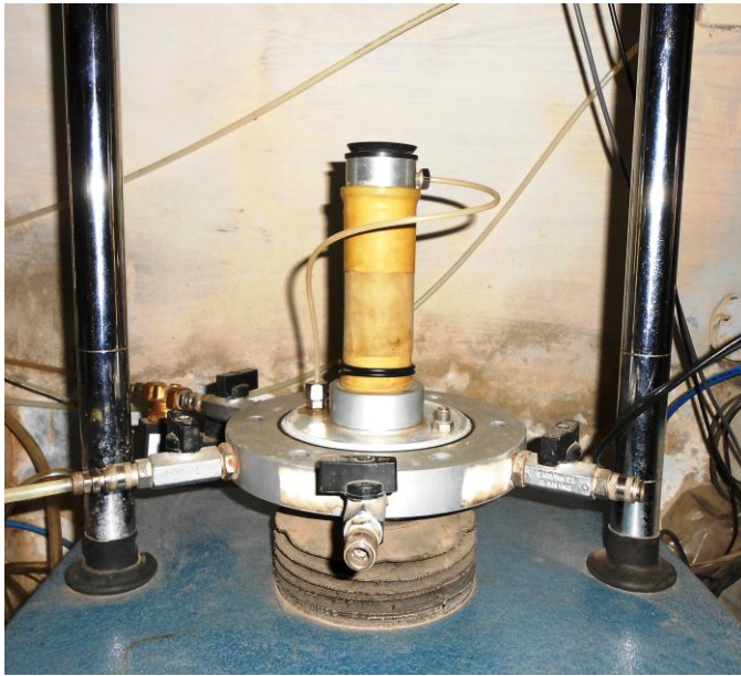
Fig. 2. A sample ready for testing on cyclic triaxial
