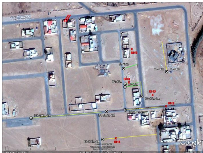
Fig.2. Borehole and electrical resistivity lines conducted.
