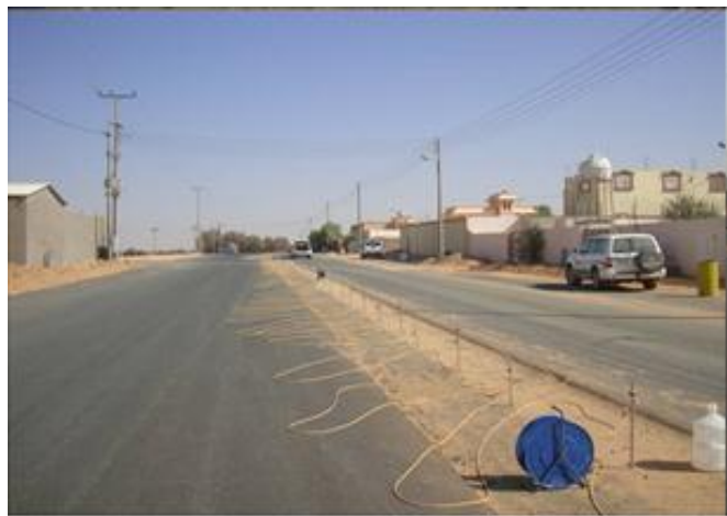
Fig.3 View of electrode distribution along one resistivity line.
