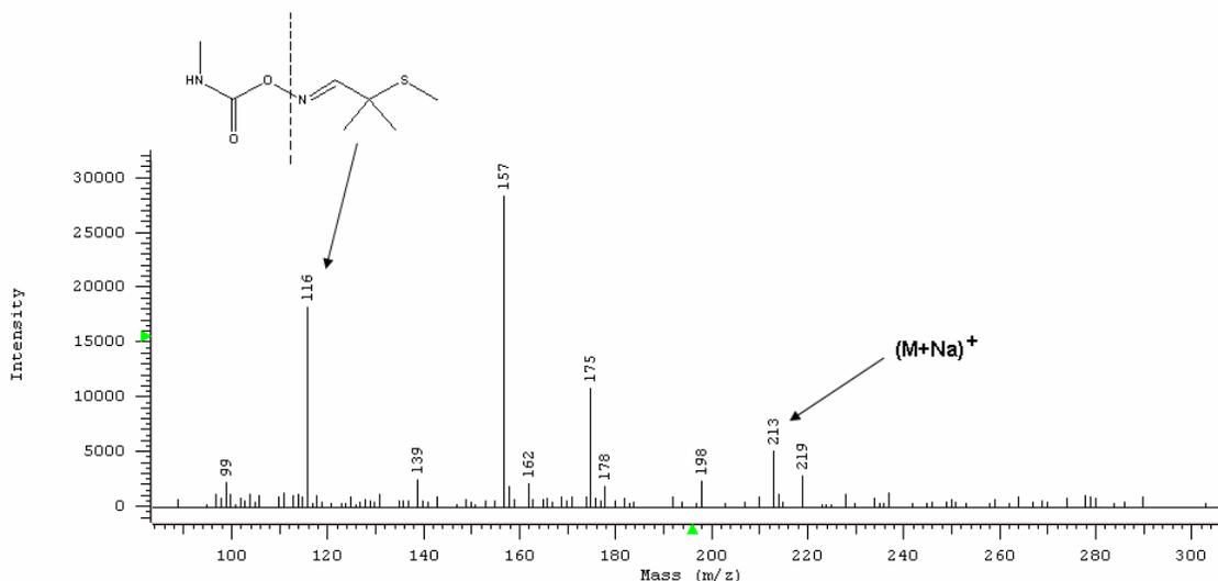
Fig. 2 - Mass spectrum of Aldicarb (MW: 190) standard
