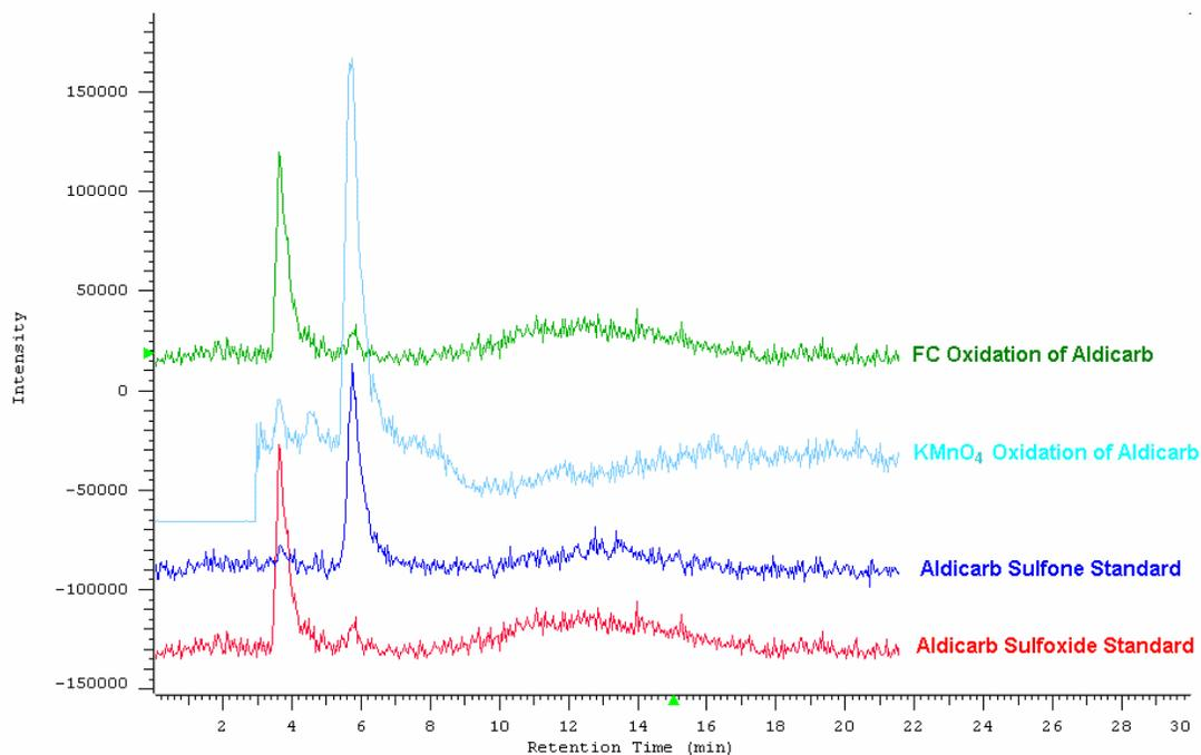
Fig. 3 - TICs of aldicarb sulfoxide and aldicarb sulfone standard, and representative byproducts of aldicarb under FC and KMnO<sub>4</sub> oxidation systems.
