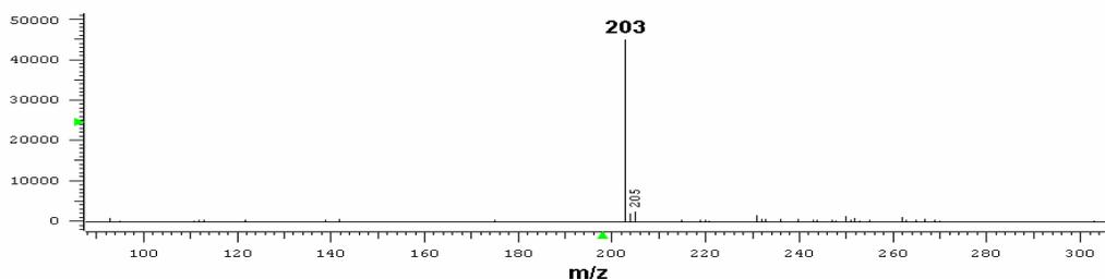
Figure 6. Mass spectrum of MS<sup>2</sup> of fonofos oxygen analog.
