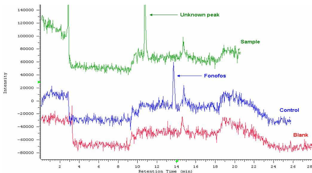
Figure 1. Total ion chromatograms of free chlorine oxidation of fonofos at pH 7.0.
