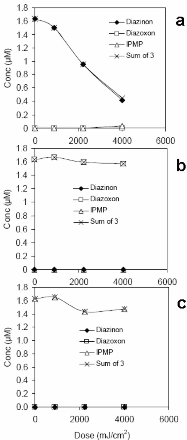
Figure 6. UV radiation profiles of (a) diazinon system (initial concentration of diazinon:  $1.64 \mu\text{M}$ ), (b) diazoxon system (initial concentration of diazoxon:  $1.63 \mu\text{M}$ ), and (c) IPMP system (initial concentration of IPMP:  $1.64 \mu\text{M}$ ).
