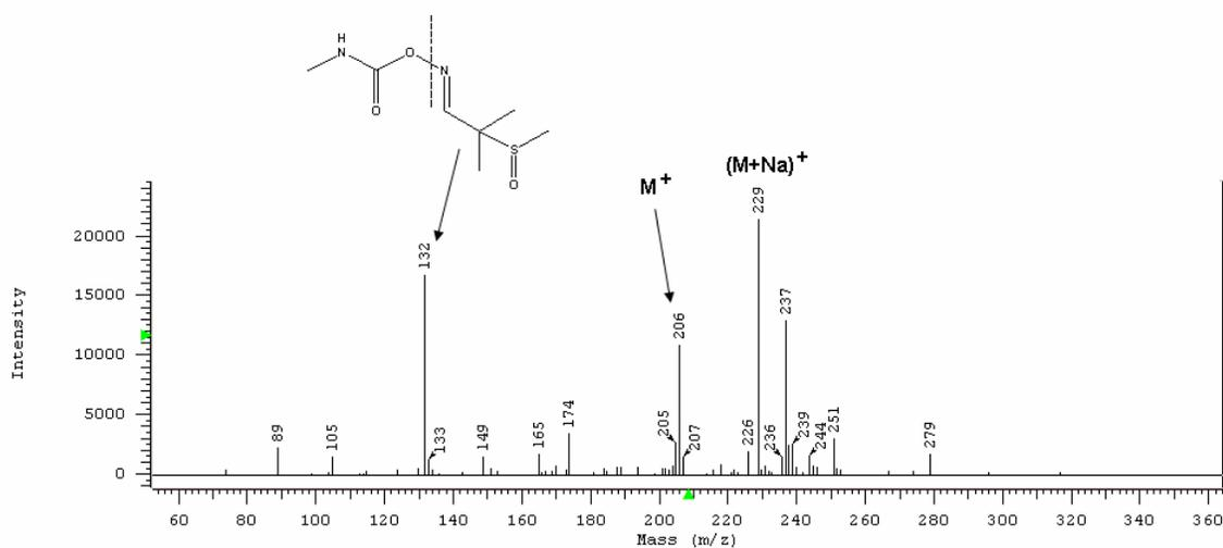
Fig. 4 - Mass spectrum of aldicarb sulfoxide (MW: 206) standard and the oxidation byproducts of aldicarb under FC, MCA, O<sub>3</sub> and H<sub>2</sub>O<sub>2</sub> oxidation systems.
