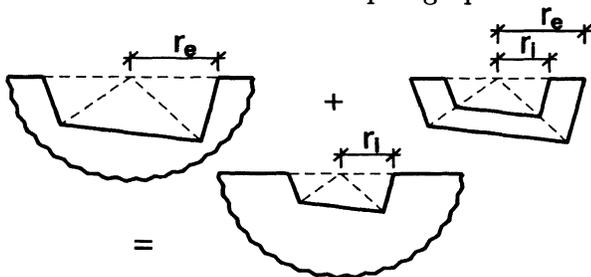
Fig. 1. Fundamental Concept of Infinitesimal Finite-Element Cell Method
