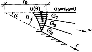
Fig. 3. Inhomogeneous Semi-Infinite Wedge with Prescribed Linear Displacement
