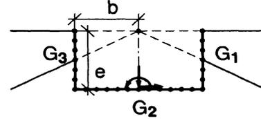
Fig. 6. Rectangular Foundation Embedded in Inhomogeneous Half-Plane
