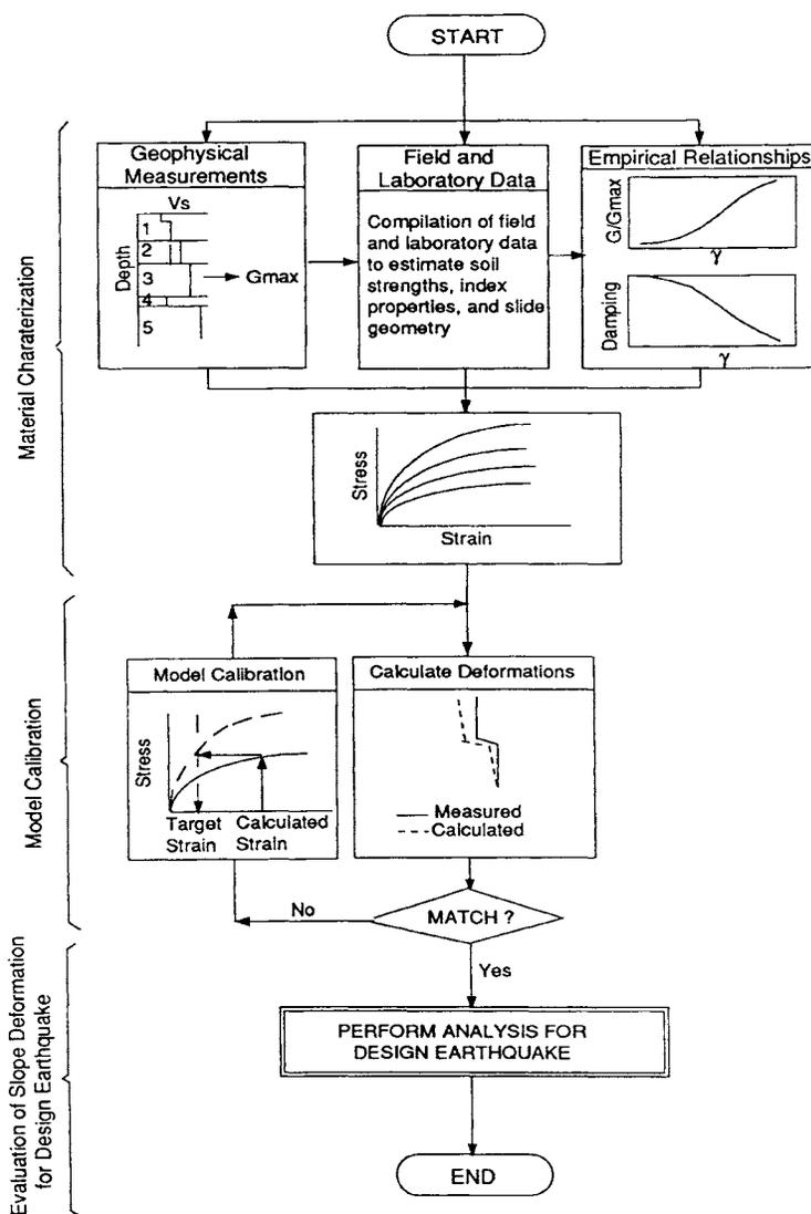
Figure 3. Methodology for the Calibration Analysis
