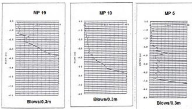
Fig. 6. Typical results of Macintosh probes at km 39
