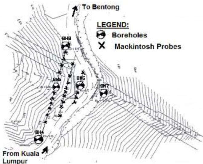
Fig. 4. Location of borehole and Mackintosh probes
