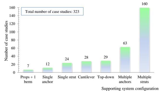
Fig. 3. Distribution of case studies based on the supporting system configuration.
