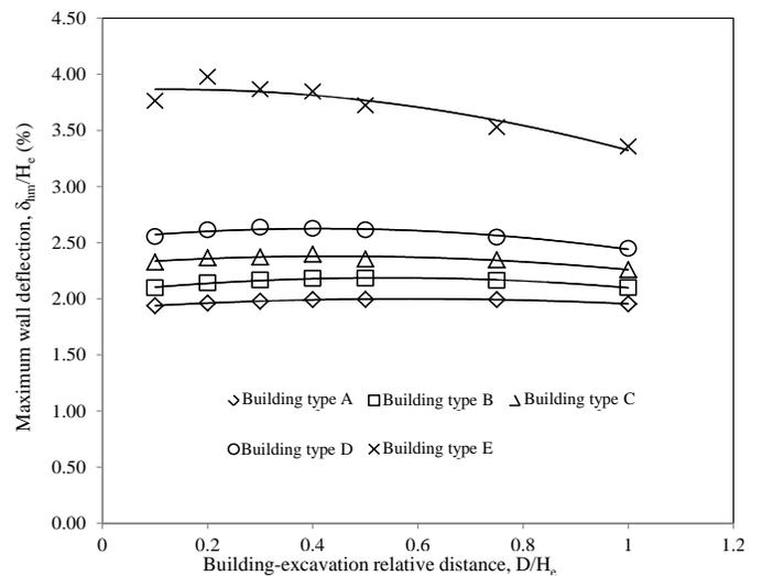
Fig. 5. Variation of normalized maximum lateral wall deflections with relative distance excavation-building.
