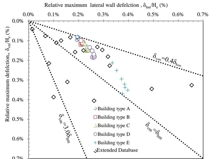
Fig. 7 Normalized maximum retaining wall deflections vs. normalized maximum settlement.
