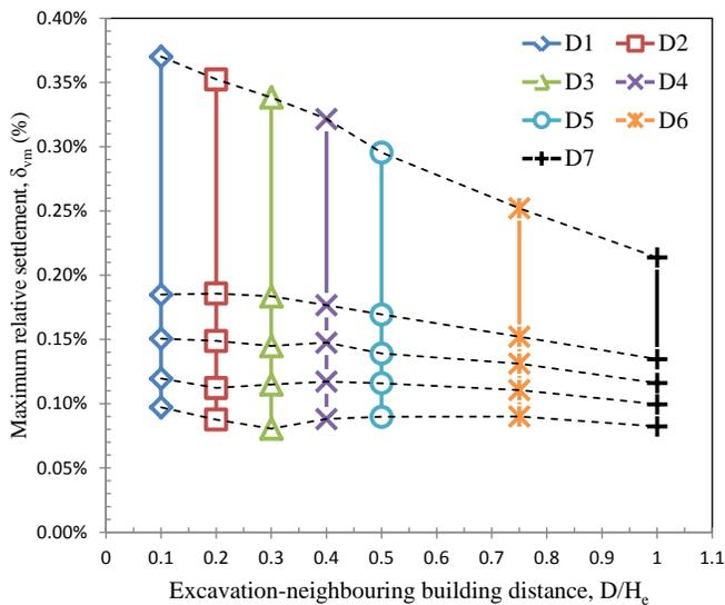
Fig. 6 Variation of neighboring buildings' normalized maximum settlements with excavation-building distance.
