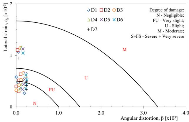
Fig. 8. Comparison of damage level for the neighboring buildings to chart of Boscardin and Cording (1989).
