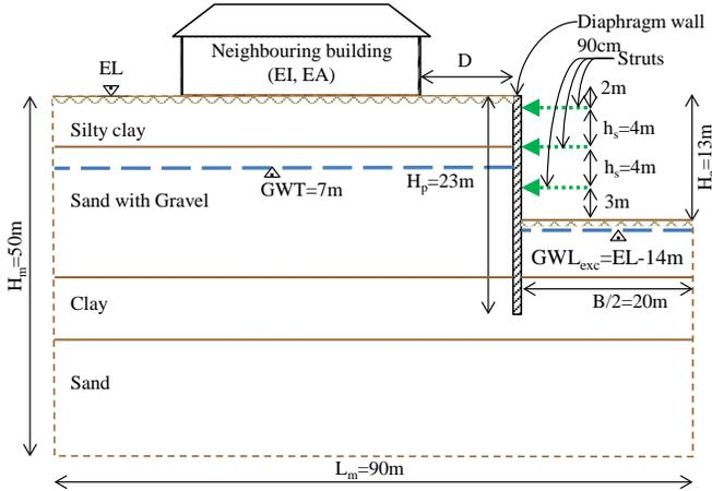
Fig. 4. Geometry of the FE model for the parametric study.
