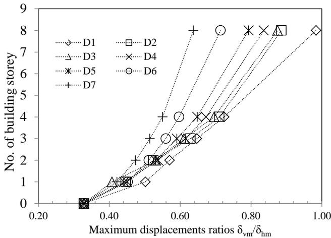
Fig. 9. Ratio of the maximum settlement and the maximum lateral deflection of the retaining wall  $\delta_{vm}/\delta_{hm}$  versus the number of stories of the neighboring building.
