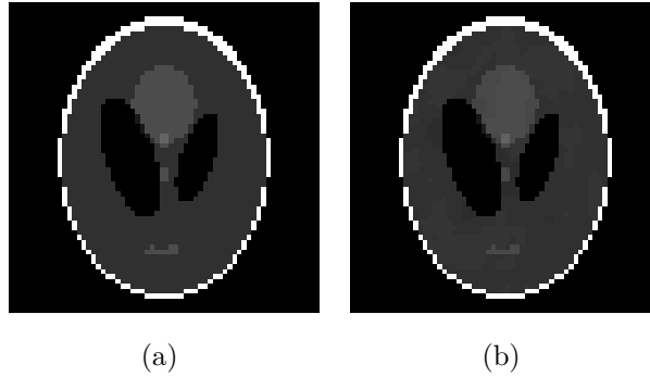
Figure 6: Shepp-Logan phantom images from complete data and recovered data from 30% randomly selected frequency points.
