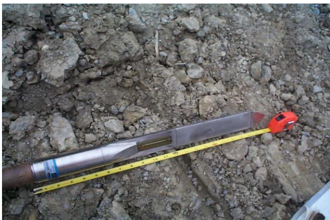
Fig. 6: Push-in earth pressure cell.
