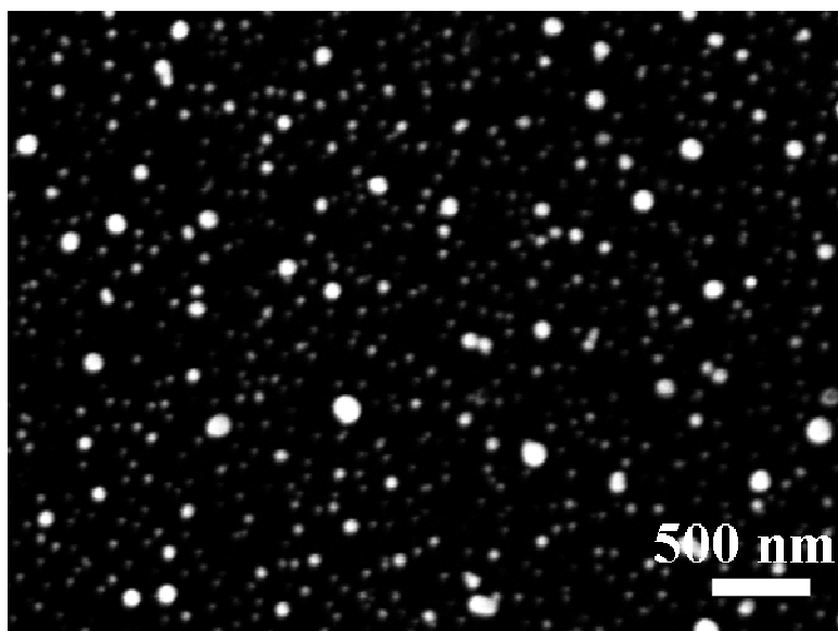
Figure 2.12 SEM image of gold particle.
