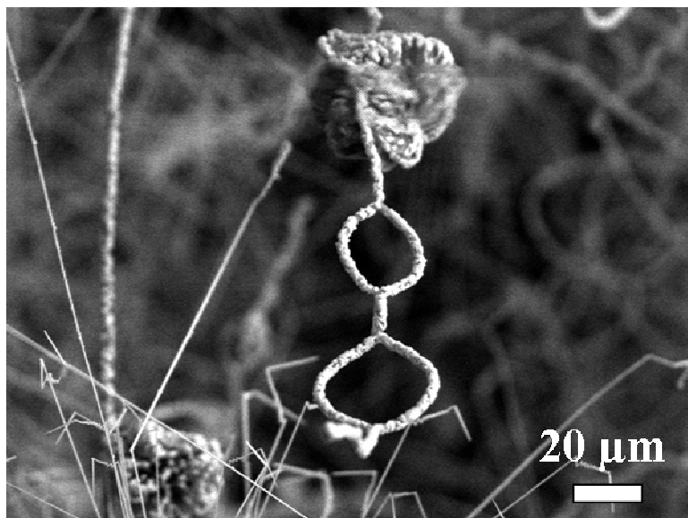
Figure 3.12 SEM image of silica “glasses”. The diameter of the glasses is around 20 micrometers (2006, J. Liu).
