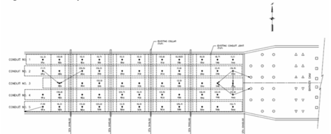
Figure 22 - Polyurethane Material Gout Volume, Barker Dam
