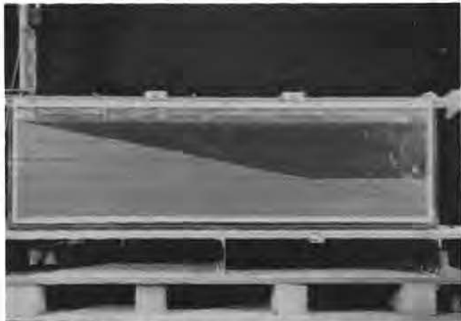
Fig.2a Shape of loose model slope prior to shaking.
