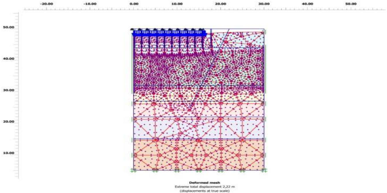
Figure 9- Distribution of vertical displacement without inclusions
