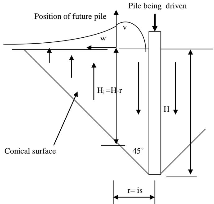
Fig.3. Soil displacements within impedance zone of pile
