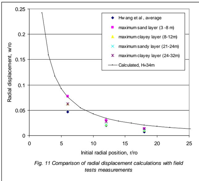
The tests involved driving precast RC piles 800 mm in diameter to depths of 34 m through layers of silty clay, (3-8m), soft clays(8-12m), medium sands(12-21m), a clay layer interbedded with thin layers of sand(21-32m) and medium dense sands(32-40m). It is instructive to look at the ability of the analytical model to predict the movements in a
