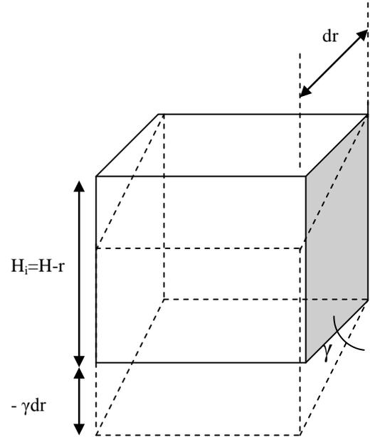
Fig. 4 Shearing of a soil element in the near field of the pile shaft
