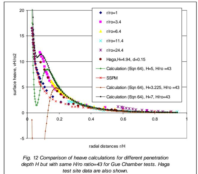
The spikes in predicted values near to the pile shaft are likely due to computation errors. Equation (64) does not predict well near to the pile shaft where  $r/H < 0.1$ . The predictions are in good agreement with the data for  $r/H$  from 0.1 to 0.2 onwards. Also plotted in these figures are the predictions by the Shallow Strain Path Method (SSPM) (Sagaseta and Whittle, 2001) which was derived using fluid mechanics and
