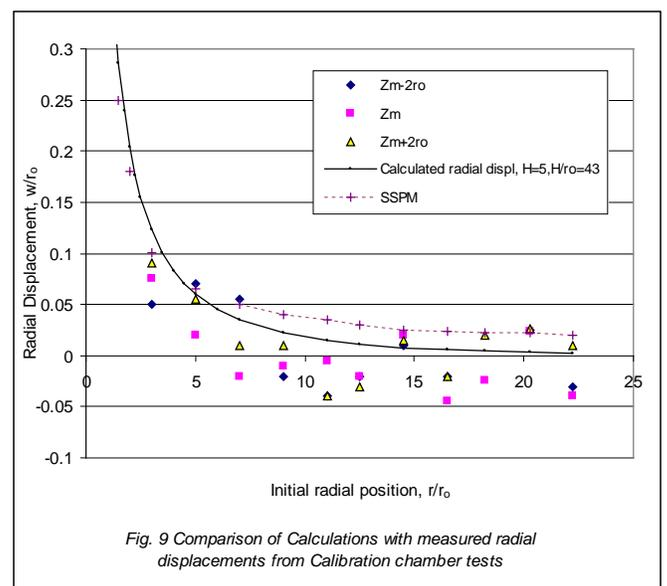
Figure 9 plots the predictions of equation (31) and that of SSPM with measured radial displacements ( $w/r_0$ ) versus the initial radial position ( $r/r_0$ ) from the calibration chamber tests of Gue. Both Equation (31) and the SSPM are in reasonable agreement with the measured radial displacements for the moderate distances except that the SSPM tends to predict higher values at far distances.
