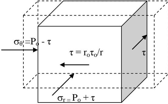
Fig. 1b. Shearing of a soil element in moderate to far distance from pile under cavity expansion.
