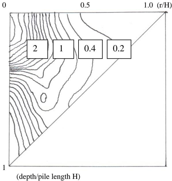
Fig.2 Contours of normalized vertical displacements within soil mass measured at Hendon based on data of Cooke and Price(1973) at all stages of driving of piles (contours adapted from Sagaseta and Whittle, 2001)
