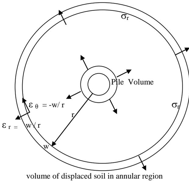
Fig.. 1a Modelling of the displacement process
