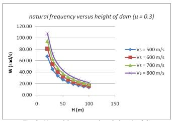
Fig. 2. Natural frequency of earth dam ( $\mu$ =0.3)
