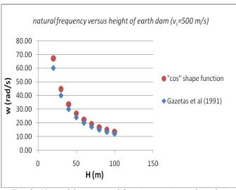
Fig. 8. Natural frequency of dam (comparison of results)
