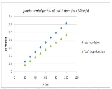
Fig. 9. Fundamental period of dam (comparison of results)
