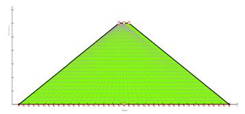
Fig. 4. Model of dam with rigid foundation
