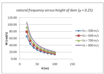
Fig. 3. Natural frequency of earth dam ( $\mu$ =0.25)
