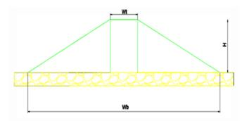
Fig. 1. Geometry of earth dam
