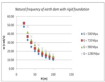
Fig. 7. Natural frequency of dam with rigid foundation
