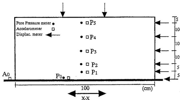
Fig.1. Schematic view of the models and instrumentation.
