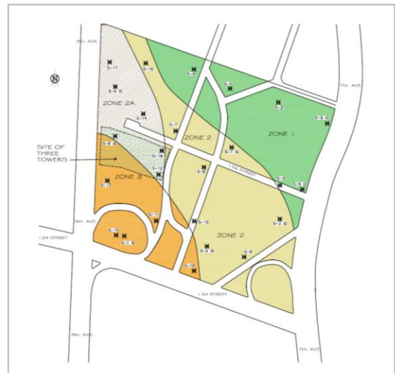
Fig. 9. Geotechnical zoning preliminary report 1996
