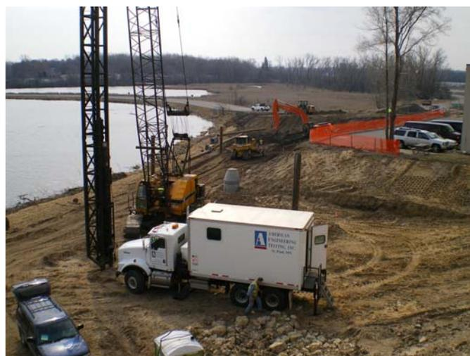
*Fig. 1. SCPTu testing at the project site.*
