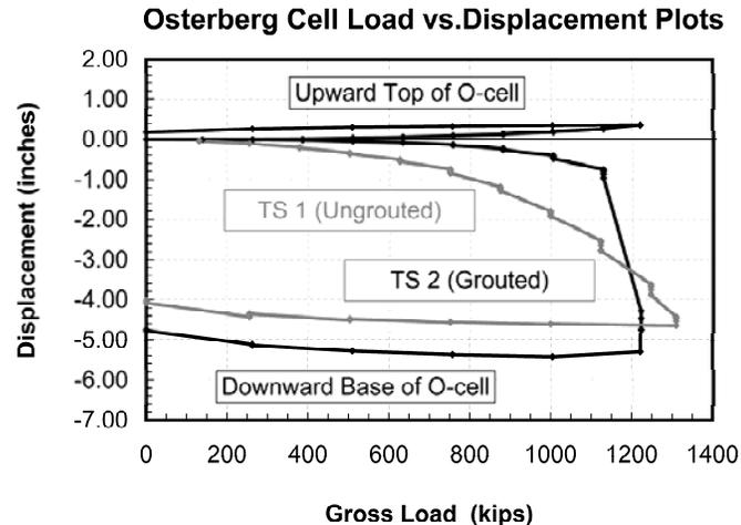
Fig. 6. Load-Movement curves for Broadway Viaduct
