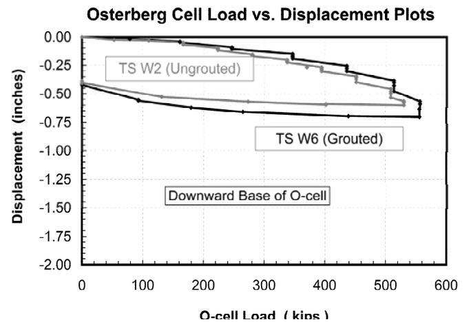
Fig.10. Downward Load-Movement Curves for Missouri Research Project
