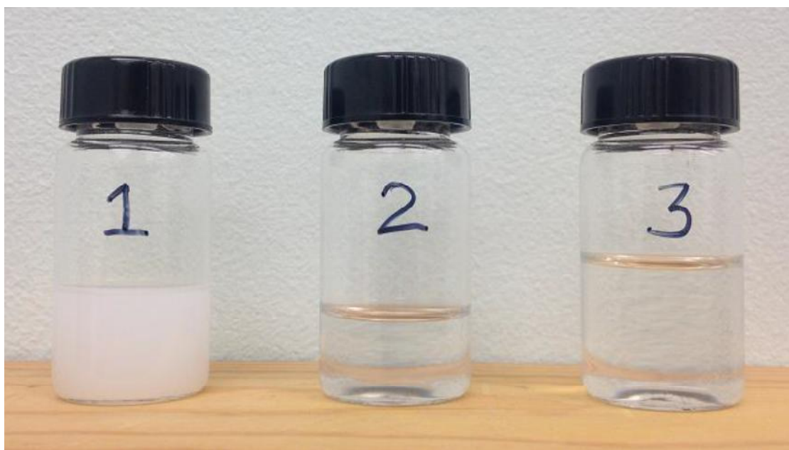
Figure 3. Vial 1: CUP solution of poly-1 before filtering; Vial 2: CUP solution of poly-1 after filtering; Vial 3: CUP solution of poly-5 (MW = 16K).
