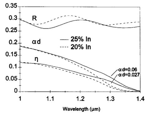
FIG. 2. Experimental reflectance ( $R$ ), quantum efficiency ( $\eta$ ), and normalized absorption coefficient ( $ad$ ) spectra of conventional *p-i-n* structures (i.e., without a resonant cavity) similar to the one illustrated in Fig. 1 with indium concentrations of 20% and 25% in the absorbing layers.
