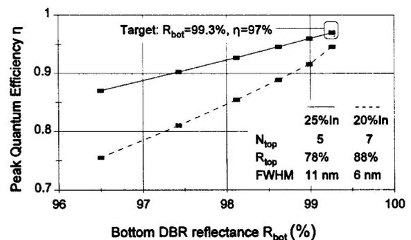
FIG. 3. Simulated peak quantum efficiency  $\eta$  at 1.3  $\mu\text{m}$  of a RCE *p-i-n* photodetector as a function of the bottom DBR reflectance using the experimental absorption values of Fig. 2.  $N_{\text{top}}$ ,  $R_{\text{top}}$ , and  $R_{\text{bot}}$  are the number of periods of the top DBR and reflectance of the top bottom DBR, respectively. FWHM is the full width at half maximum of the peak quantum efficiency.
