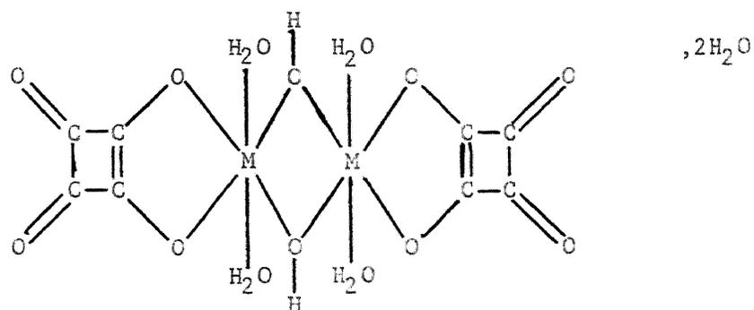
Figure XII. Proposed Dimeric Structure of Trivalent Metal Squarate Trihydrates
