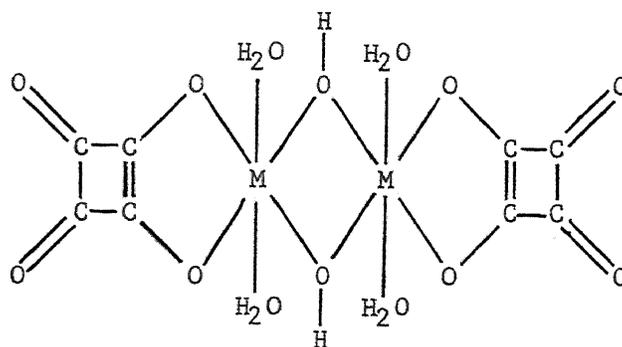
Figure XIV. Proposed Dimeric Structure of Trivalent Metal Squarate Dihydrates
