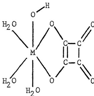
Figure XI. Proposed Pseudo-octahedral Structure of Trivalent Metal Squarate Trihydrate
