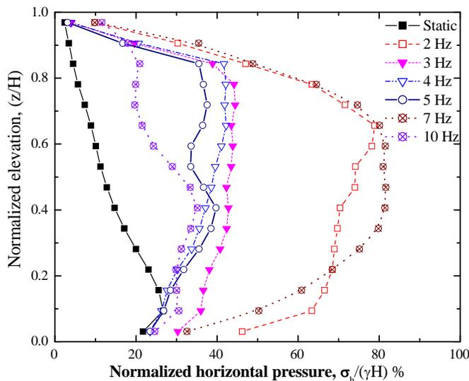
Fig. 12 Seismic earth pressures at different frequency levels
