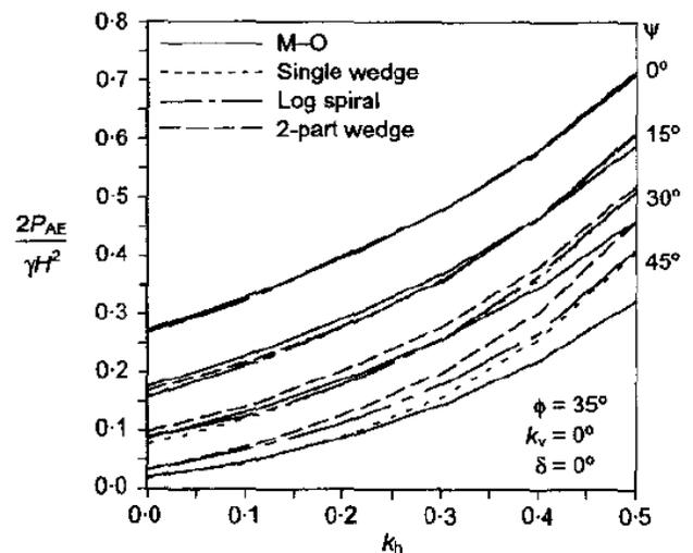
Fig. 2 Comparison of wedge and log-spiral failure surface pseudo static methods (after Bathurst et al. 2002)
