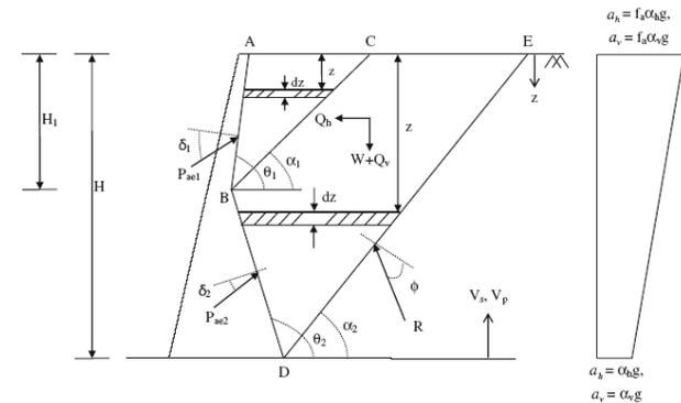
Fig. 4 Geometry and forces considered in pseudo-dynamic method for the analysis of a bilinear wall (after Kolathyar and Ghosh 2009)
