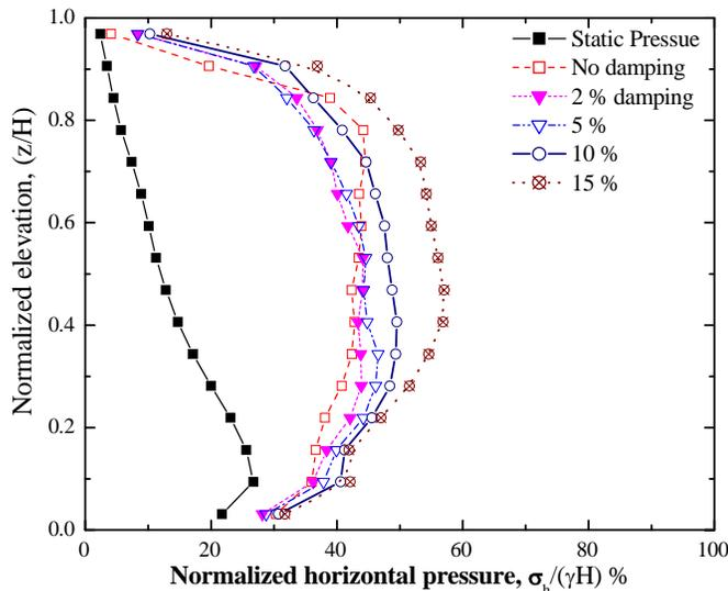
Fig. 13 Seismic earth pressures at different damping levels
