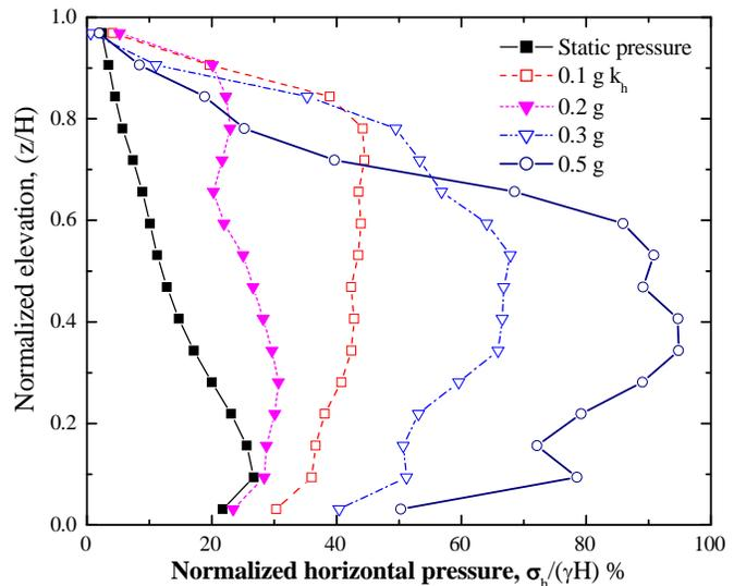
Fig. 11 Seismic earth pressures at different acceleration levels
