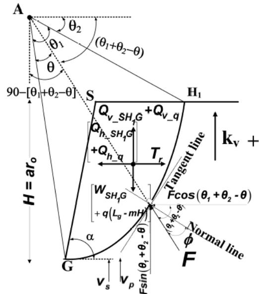
Fig. 3 Geometry and forces considered for log-spiral failure surface (after Basha and Babu 2009b)
