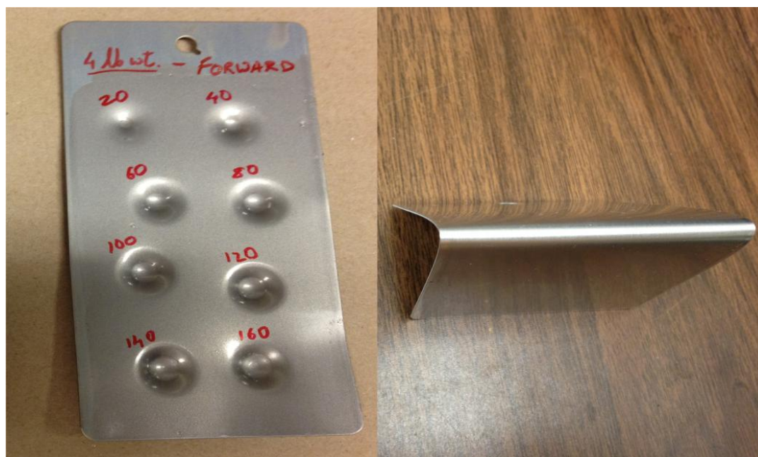
Figure 11. High impact resistance and flexibility of melamine cured CUP clear coatings.
