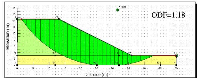
Fig. S13 Same material parameters as in Fig. S12, different definition of failure surface. Geo-Studio input file: Part_B_StageII_UniformAlluviumCircle.gsz ]
