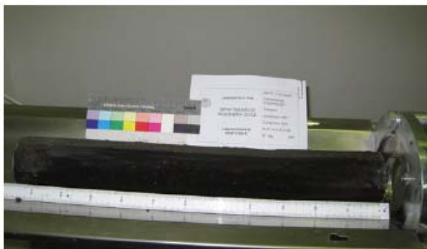
Fig. 5.c. Example of a good quality odometer test: picture of tested sample (borehole S1, sample C3).
