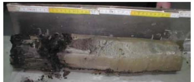
Fig. 6.b. Example of an odometer test using a sample of low quality: picture of tested sample (borehole S1, sample C4).
