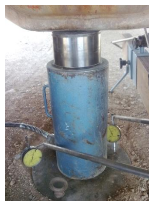
Fig. 5 Plate load testing at the semnan university campus, Iran.
