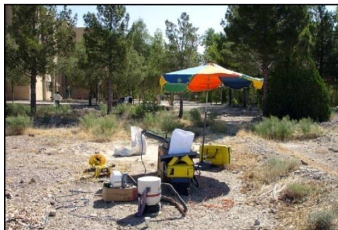
Fig. 4 Small-strain stiffness measurements at the semnan university campus (Iran) using continuous surface wave system
