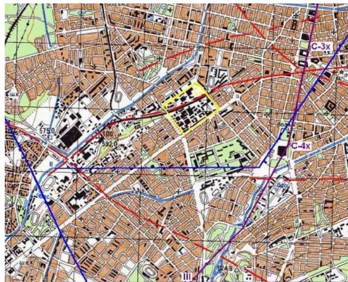
*Fig.3. Urban plan of the central part of Sofia City with indicated area of the site (the yellow square). The red lines are the known faults. The blue lines are the profiles of special studies of the seismic properties of the geological grounds*
