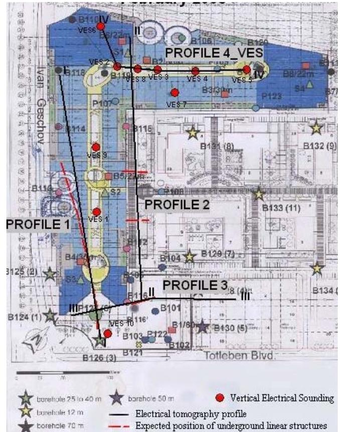
Fig. 5. Situation with the position of the measurement by the method of VES and the profiles of electrical tomography investigation.
